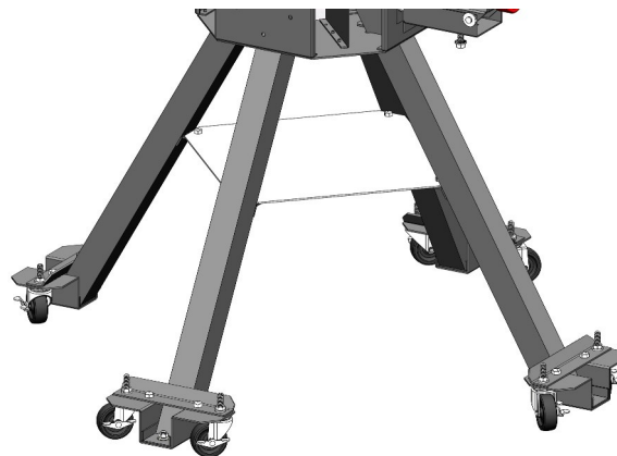
Drop Down Wheel Set Installed
